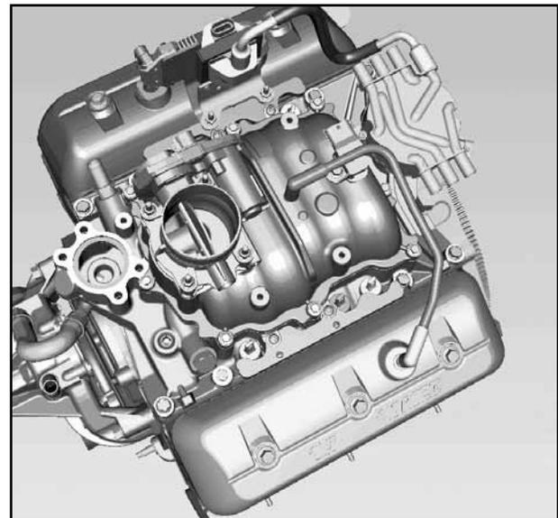
*The Integral Air Fuel Module (IAFM) incorporates several components into one assembly. The bottom of the inlet manifold is made of iron and the top is made of aluminum. Integrated into the module is an electronic throttle body. Also included is a combination manifold absolute pressure (MAP) and manifold air temperature (MAT) sensor.*
