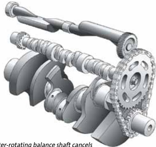
*A counter-rotating balance shaft cancels the primary engine vibrations found in 90° V-6 engines. The result is smooth performance and low noise.*
